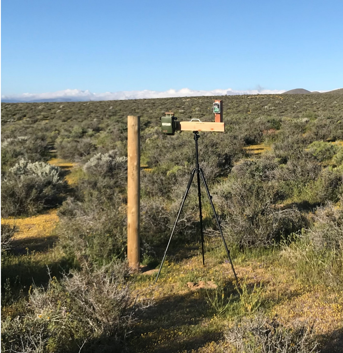
Figure 1. ARU tripod deployed at a Habitat Monitoring System sampling point at Onyx Ranch SVRA in eastern Kern County. Photo courtesy of Shane Emerson.
